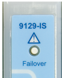
Figure 5.1: SAM failover switch
