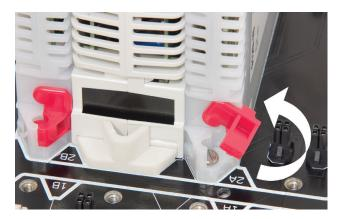
**Note:** If a FISCO power supply module position is left vacant it will cause an alarm condition to be signalled at the Alarm contacts. To prevent this a 9127-BLK blanking module can be fitted in the position normally occupied by the associated SAM module. See Section 4.2.1 for further details.
