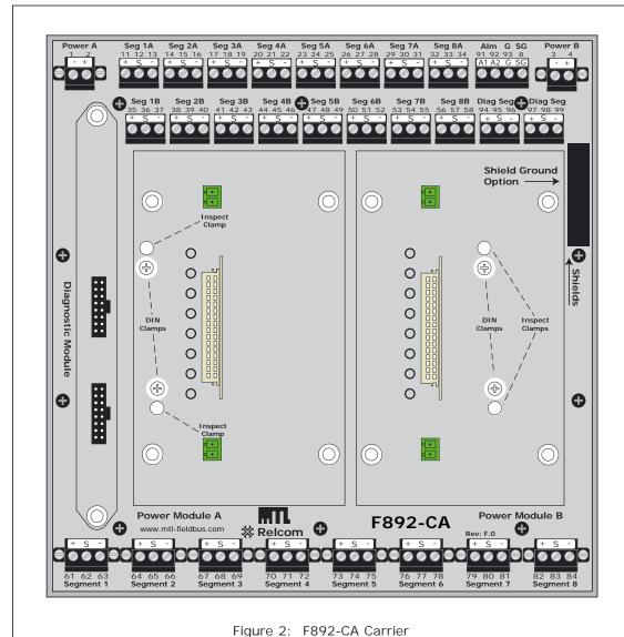
Carriers with date codes 0711 or earlier are only provided with a single row of eight connectors (top). The Diagnostic Segment Connectors were introduced on carriers with date codes after 0726. The Shield Ground Option was added with revision F.0 (previous version did not carry a revision). See sections 5.4, 5.6, and 5.8 for further details.
