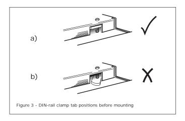
Press the carrier onto the DIN-rail and rotate each of the **DIN clamp** screws clockwise until the tab tightens against the DIN-rail. The clamping tabs can be seen through the **Inspect clamps** holes when they are in the correct position.
