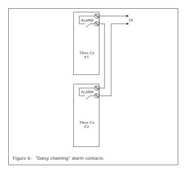
If multiple F892 units are used, a common alarm circuit can be achieved by 'daisy-chaining' the alarm circuits (see Figure 6).
