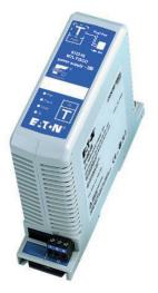
The MTL 9122-IS is a fieldbus repeater isolator which repeats the fieldbus signal from a safe area, Zone 2 fieldbus to an intrinsically safe fieldbus for connection to devices in Zone 1. The 9122-IS provides up to 256mA, typically powering up to 16 x 15mA field devices in Gas Group IIB.
