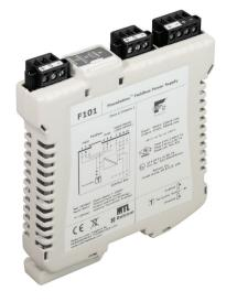
The F101 and F102 fieldbus power supplies are designed to provide power for a single FOUNDATION™ fieldbus H1 segment. Galvanic isolation, power conditioning and segment termination are incorporated into each F101 or F102 module. Termination of the fieldbus segments is normally enabled with a switch on the module, but may be switched off for those few applications that do not require a Terminator at the Fieldbus Power Supply.
