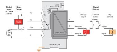
The MTL4-BSISR, for IS field devices or MTL4-BSGPR, for non-IS field devices, is used with the MTL4-ADIO isolator for digital output applications where a relay contact is required. Normally open (NO) and normally closed (NC) contacts are provided. Inductive loads must be suppressed.
